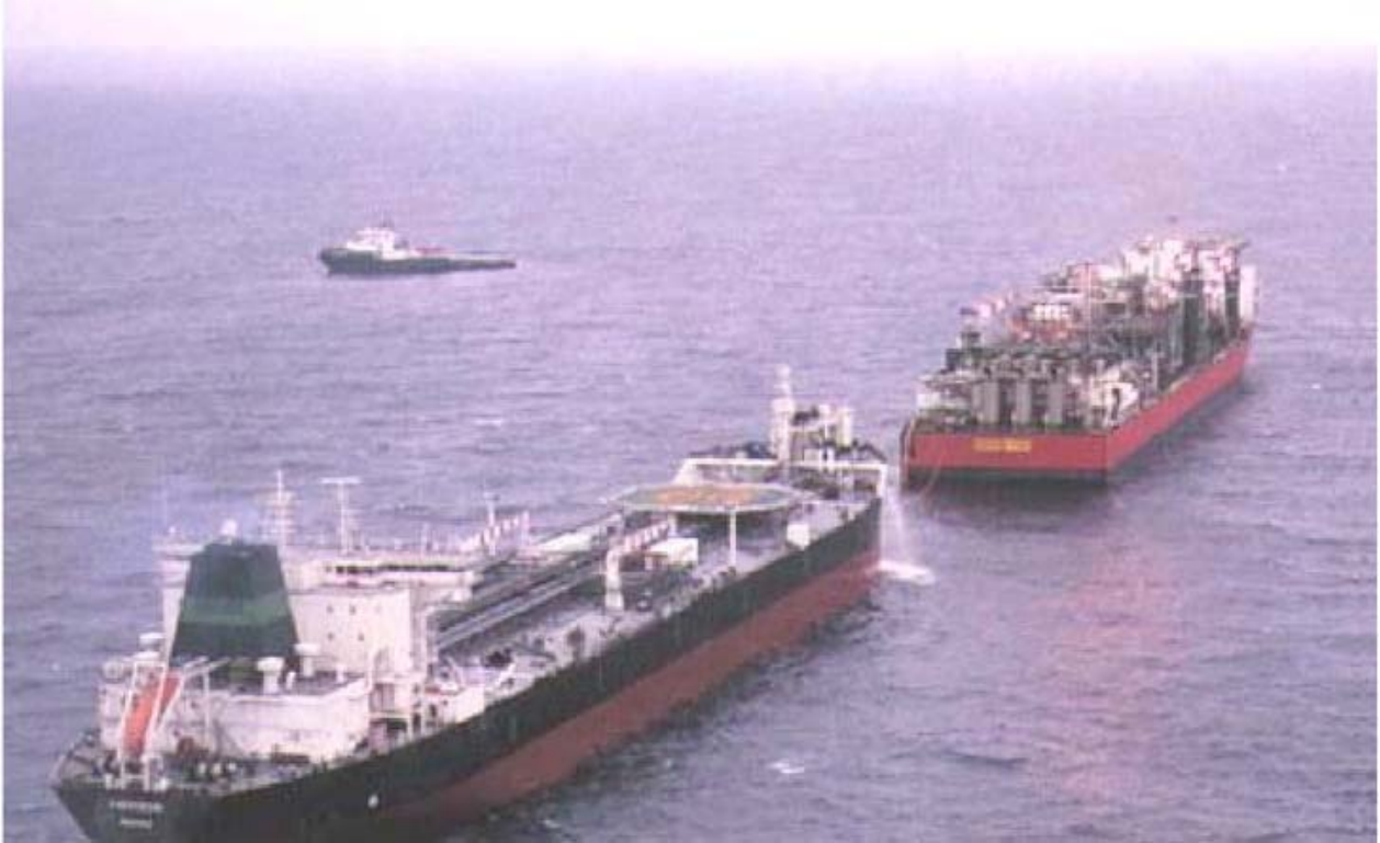
Figure 1-2 : Offloading of a FPSO by shuttle tanker and tugs
