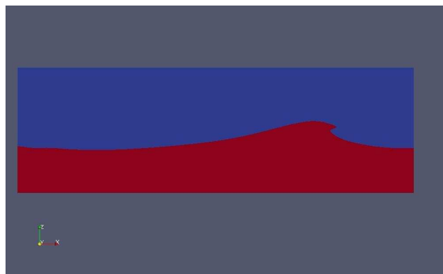
Figure 5.7: Breaking wave, earlier than expected, H = 13.36m , T = 12.31s , d = 25m , H/L = 0.074 and H/H_{max} = 0.81 , for a Stream function wave.
