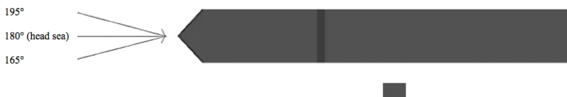
Figure 4.2: Wave directions with respect to vessel
