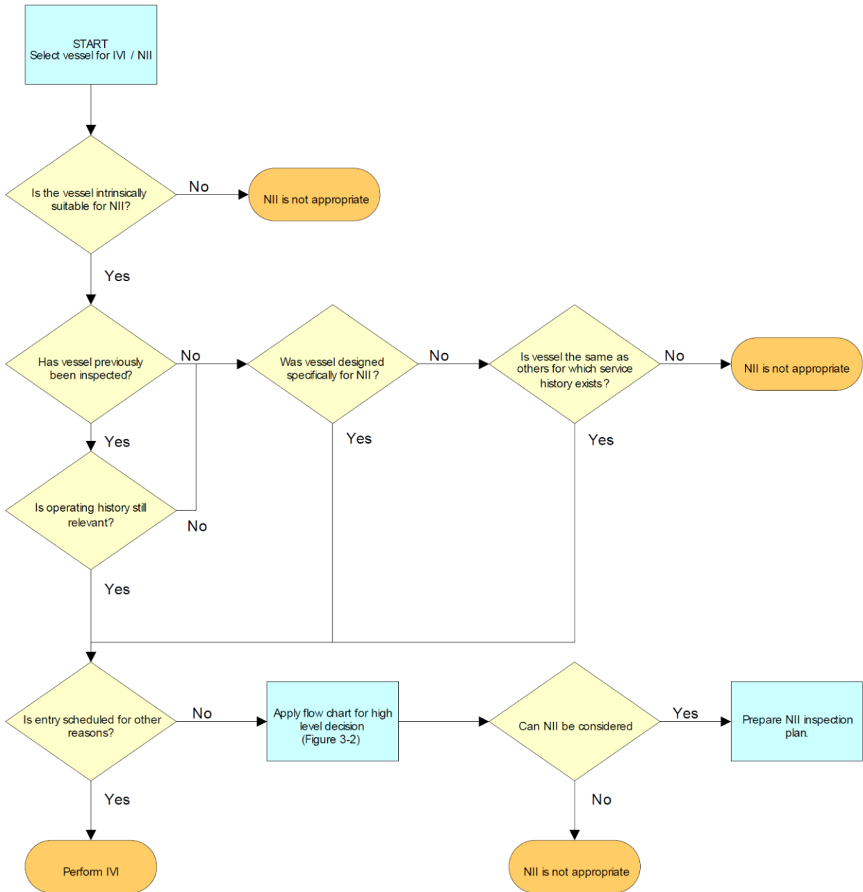
Figure 2-2: The NII preliminary screening procedure, where each questions answered leads to the final recommended decision (DNV, 2011).
