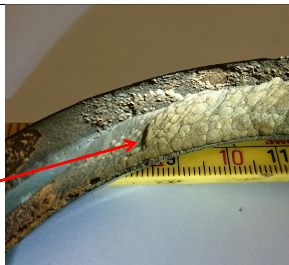
Picture G-2: RTJ - primary sealing surface 100% corroded and 50% of RTJ - secondary sealing surface after 3 years in service.
