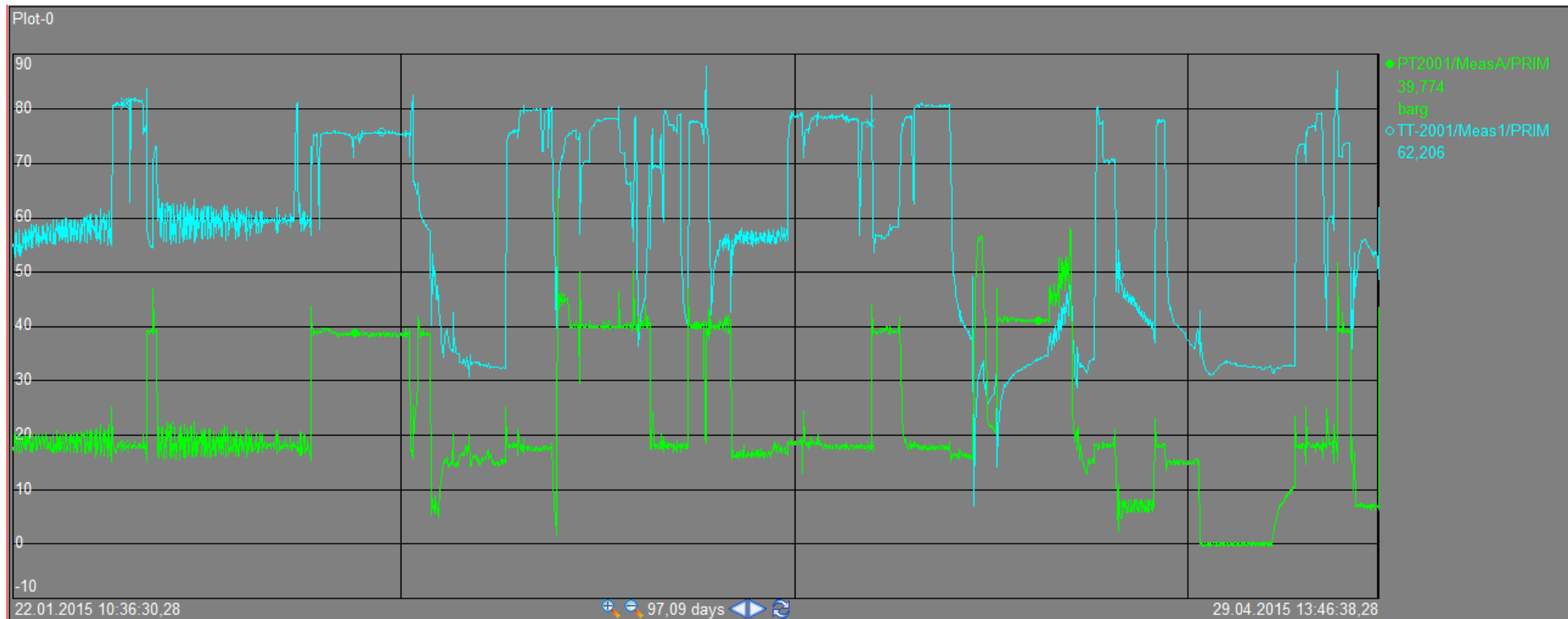
Chart C-3: Trending of the temperature and pressure in the test separator (CD2018) in a period of 97 days. The light blue line indicates the temperature in degrees of Celsius, and the green line the pressure in barg (PI Processbook, 2015).
