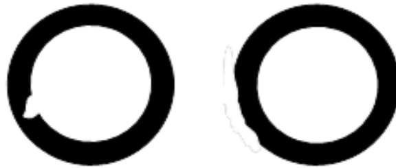
Figure 4.4.1 Pipe Loss Corrosion Section
