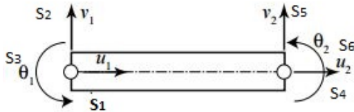
Figure 9: Degrees of freedom in a beam
