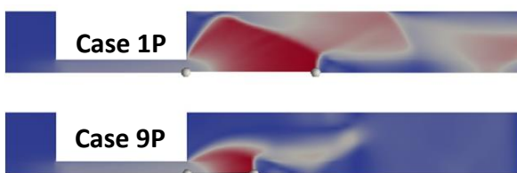
Figure 5-21 Smaller jet and less wall interaction for case 9P compared to 1P
