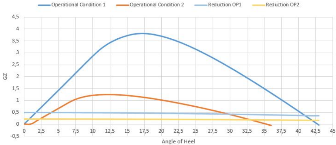
Figure 5.8: GZ curves and reductions from heeling moments
