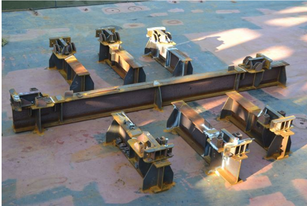
Figure 2.4: Grillage for load distribution
