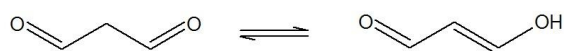
Figure 2-2 The MDA molecule in its keto and enol form. IUPAC name: propanedial.
