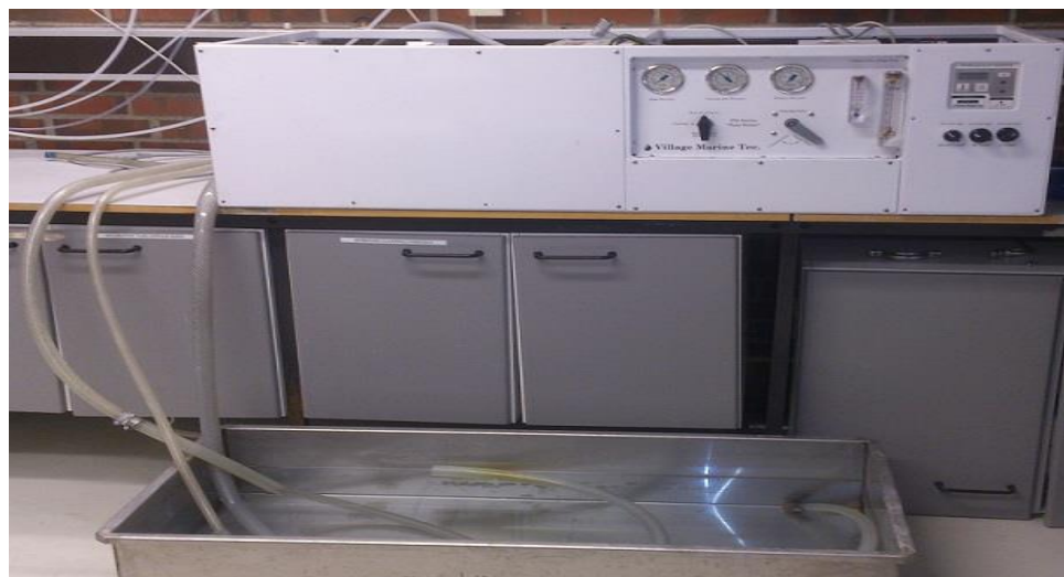
Figure 3.4 Membrane unit, feed tank and feed, permeate and retentate pipes
