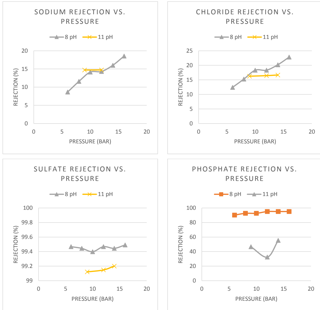
Figure 4.25 Rejection rates of sodium, chloride, sulfate and phosphate as functions of pressure at to different pH
