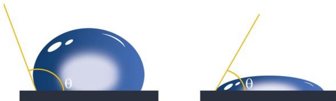
Figure 2.2 Schematic of surfaces wettability towards a liquid droplet. A surface with low wettability (left), a surface with high wettability (right).
