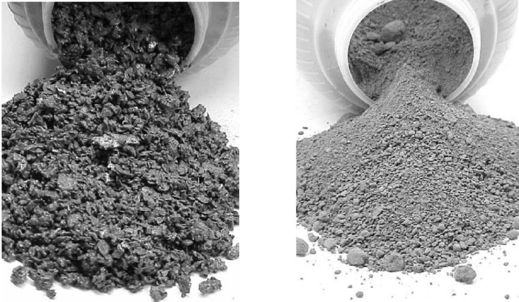
Figure 17: Cuttings prior to the treatment contains 10 percent ROC as illustrated in the picture to the left. The picture on the right side is after treatment. The ROC is reduced to 2 percent (American Society of Mechanical Engineers. Shale Shaker, 2005)
