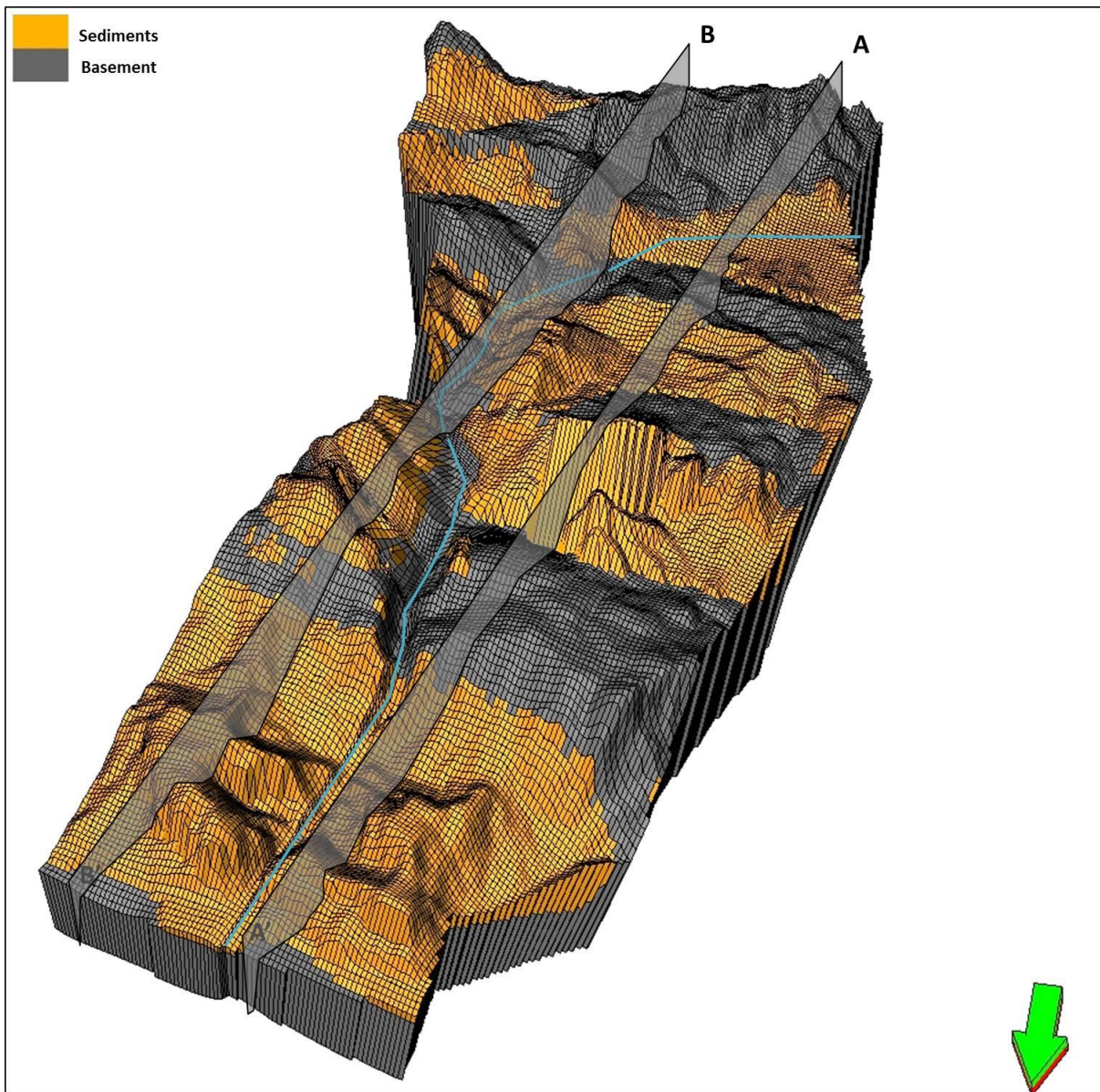
Figure 45 – 3D model representing basement (grey), sediments (orange) and the Vouraikos River (blue line), with two marked cross-sections, A and B.
