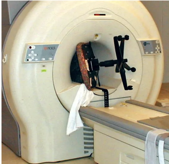
Figure 4: A picture showing a metal stool that has flown through the air into the bore. Photo by Moriel NessAiver via The New York Times[8].
