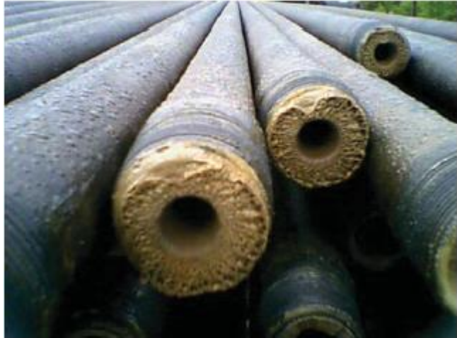
Figure 3: Barium sulphate scaled-up in tubing (Bellarby, 2009)
