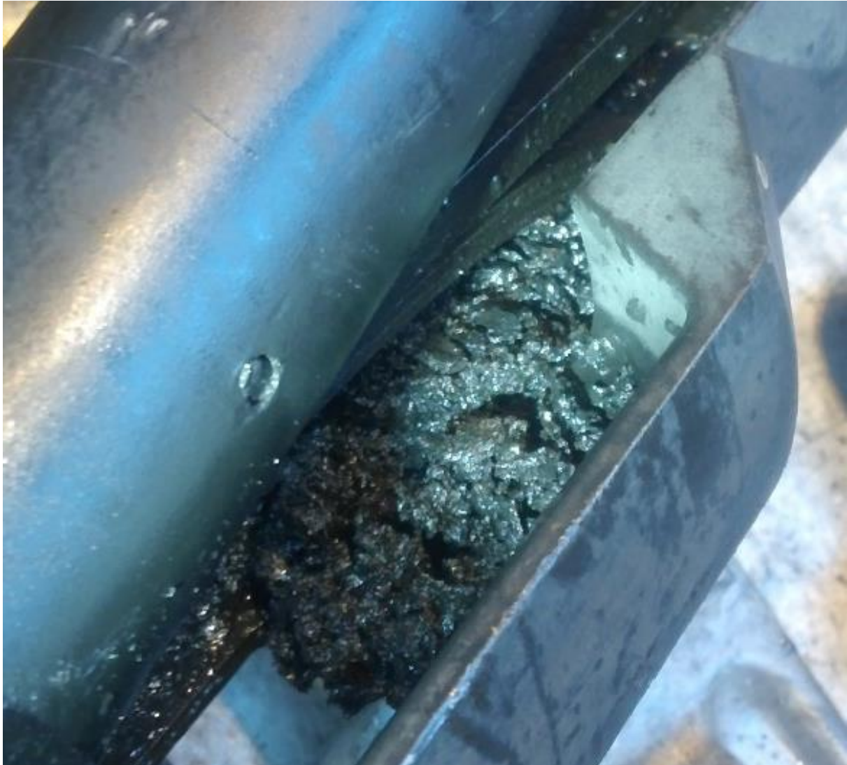
Figure 18: black sticky stuff in the kick over tool
