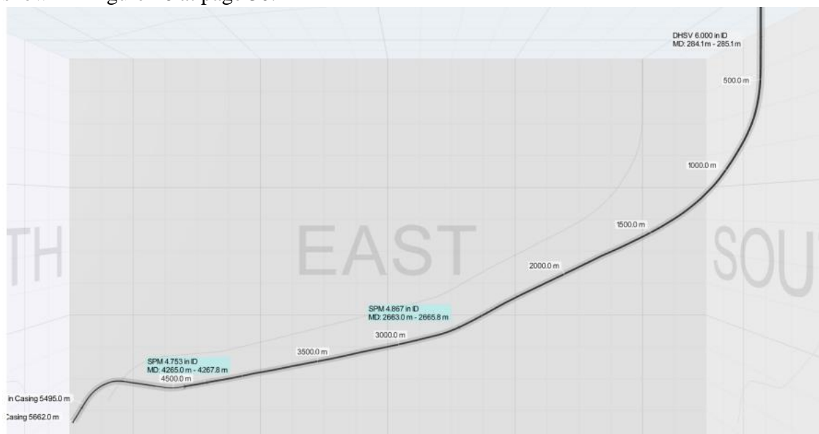
Figure 14: Well survey well X-1
