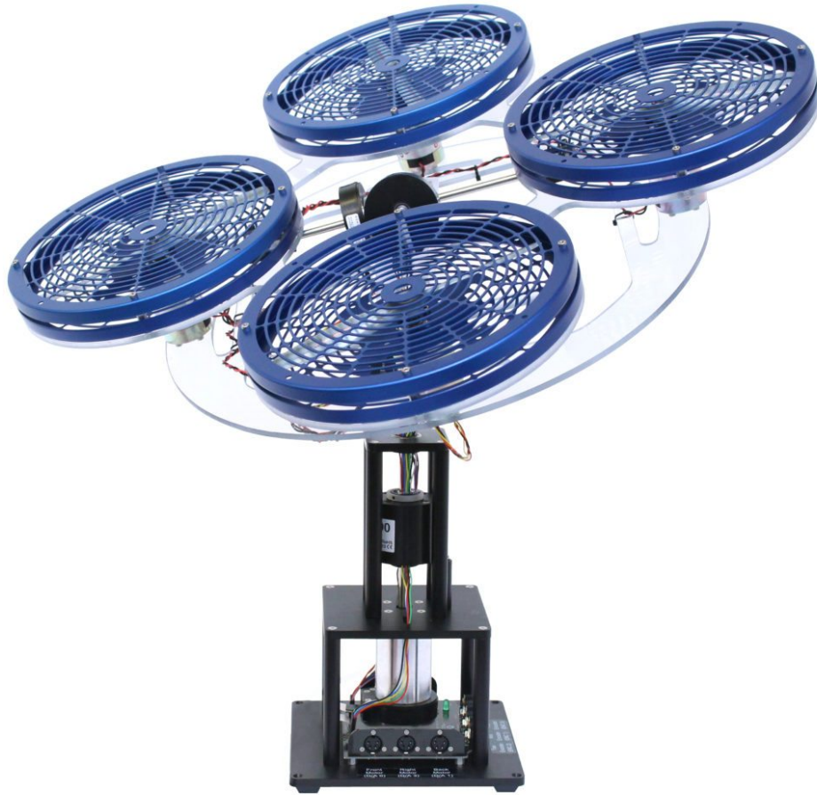
Fig 2.1: The Quanser 3DOF hover test bed.
