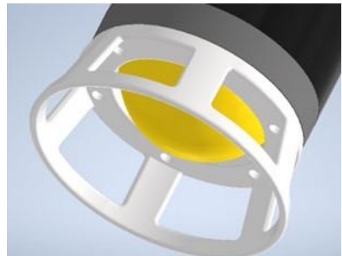
Figure 6-14 Improvement of the bladder design
