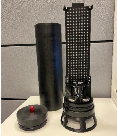
Figure 6-7 The Float and its inside structure
