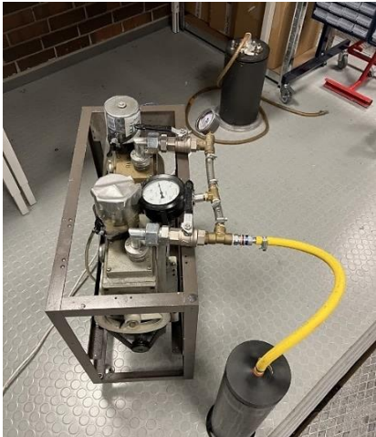
Figure 6-8 Vacuum test of the float
