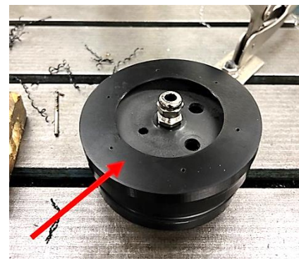
Figure 5-20 Hole transfer template
