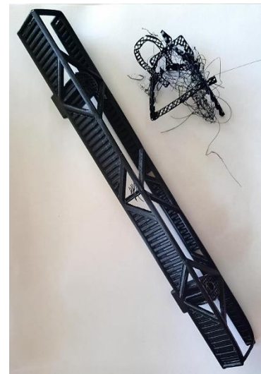
Figure 6-6 Failed 3D prints
