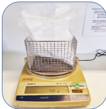
Figure 13. Figures of the procedure for thermal inactivation of spores in minced meat sample. 100 gr of the minced meat was mixed with spores (A). 6 g of minced meat containing spores was packaged, sealed, and attached to a metal rack for the heating process (B). After heat treatment, 4 g of the heated sample were transferred to a stomacher bag (C) and mixed with 36 ml of 1% peptone water using a stomacher machine.
