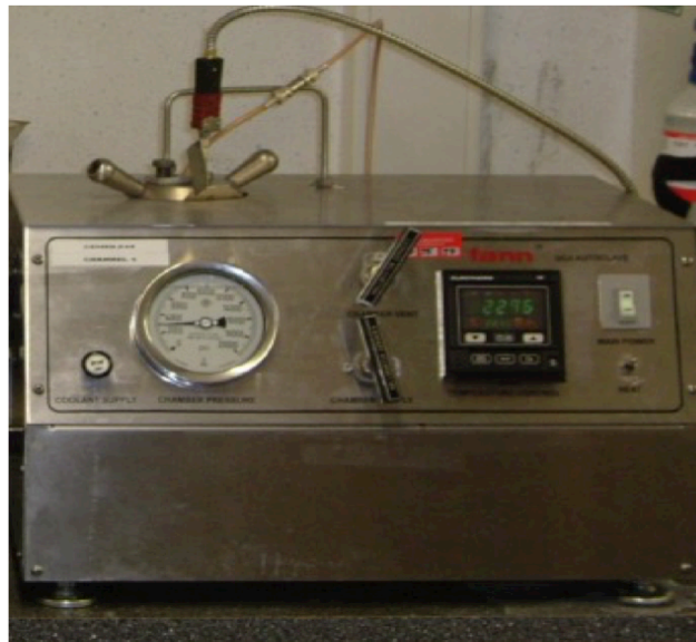
Figure 3: UCA, Halliburton cement testing lab [26]
