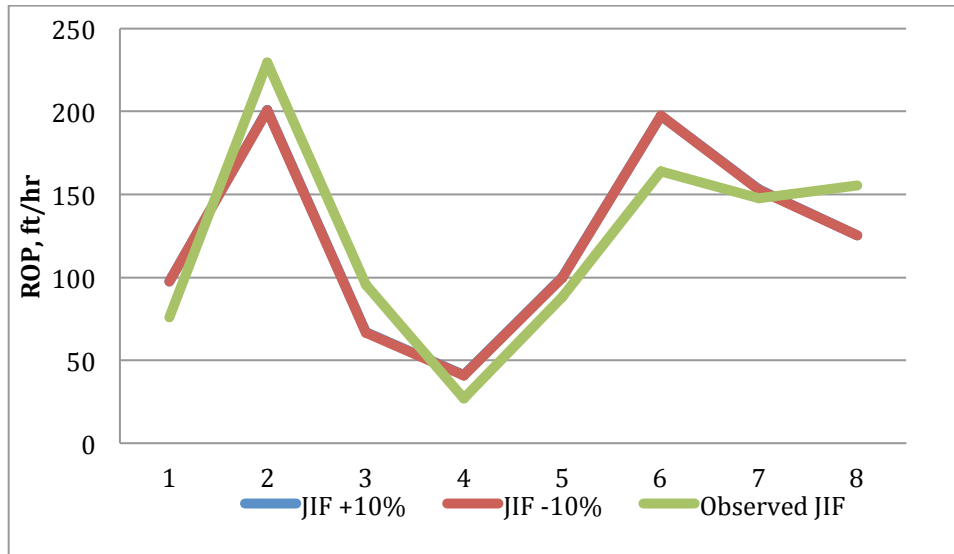
Figure 62: Effect of jet impact force variations on ROP
