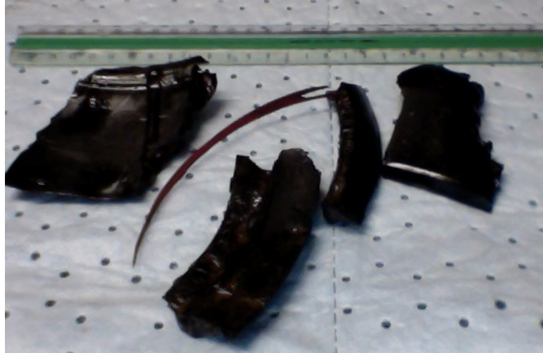
Figure 38: Rubber and plastic parts of wiper plugs, recovered on the surface 8
