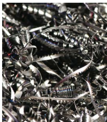
Figure 43: Collection of swarf (Halliburton)
