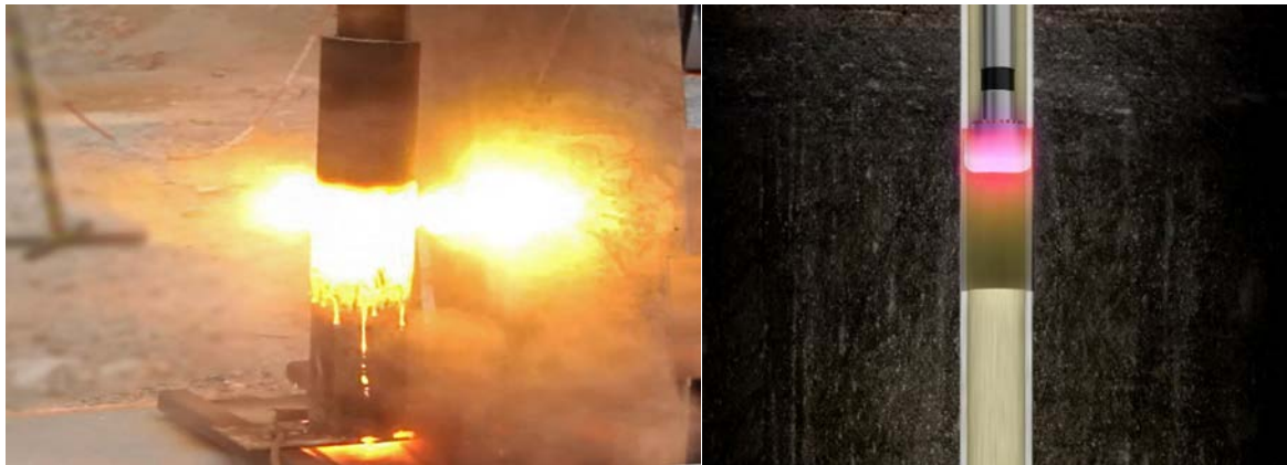
Figure 69: PLASMABIT Milling(GA Drilling, 2015)
