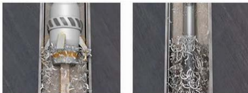
Figure 64: Reverse section milling (West Group)
