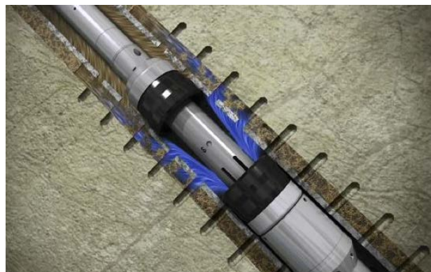
Figure 55: HydraWash Animation (HydraWell Intervention, 2015)
