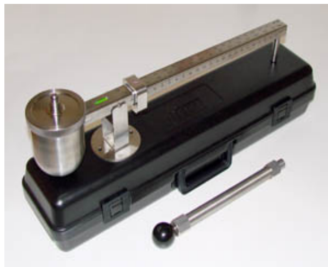
Figure 31: Photograph picture of density measuring equipment
