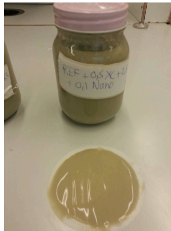
Figure 43: Mud cake from fluid system with 0.1g nanoparticles
