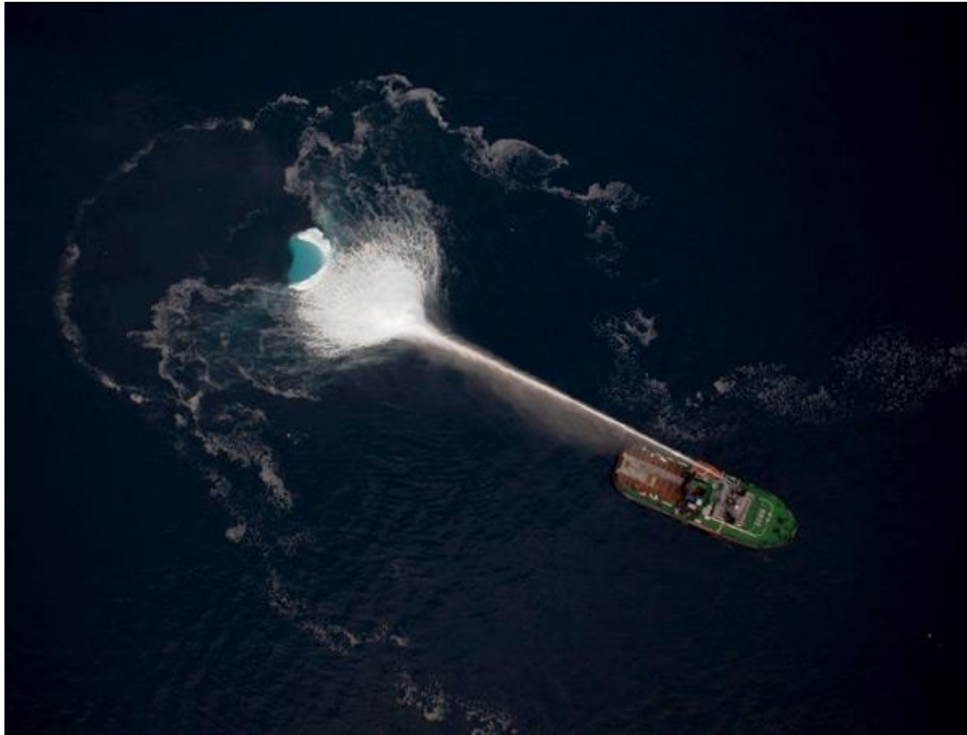
Figure 28 - Small iceberg deflected by powerful water cannon [96]
