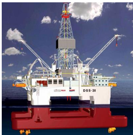
Figure 12 - Column-stabilized semisubmersible unit [32]
