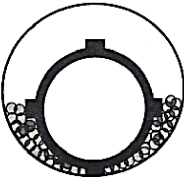
Casing - Running casing will require a cleaner hole than drilling to avoid ploughing through cuttings beds
