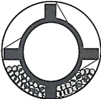
Stabilizers - can have a significant impact on how clean the hole must be to trip
