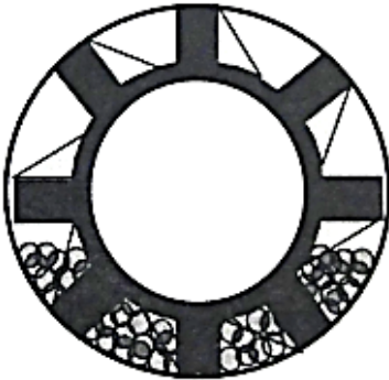
Bits - a bit with a large junk slot area will trip more freely than a heavy set bit
