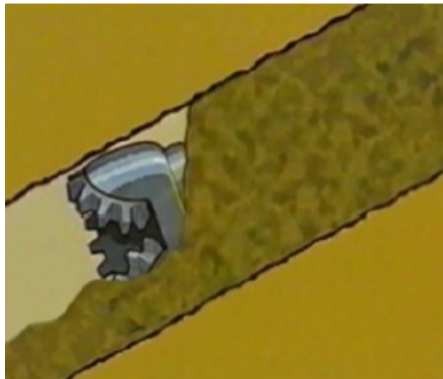
Figure 4.8: Illustration of pack-off caused by poor hole cleaning [26]
