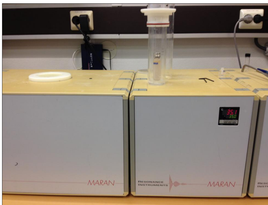
Figure 4-1: Maran Ultra NMR spectrometer (Oxford Instruments). [P1]
