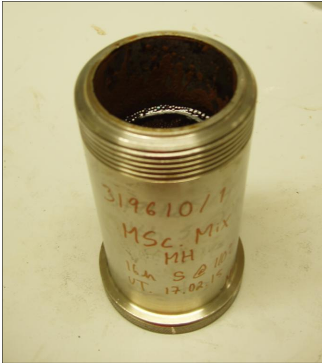
Picture 7: Freshly opened ageing cell with free fluid on top. [P1]
