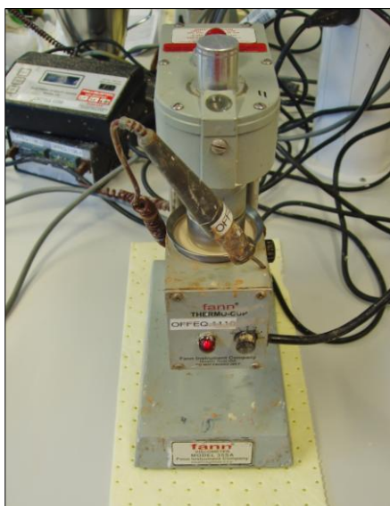
Picture 5: Fann Viscometer Model 35 SA. [P1]
