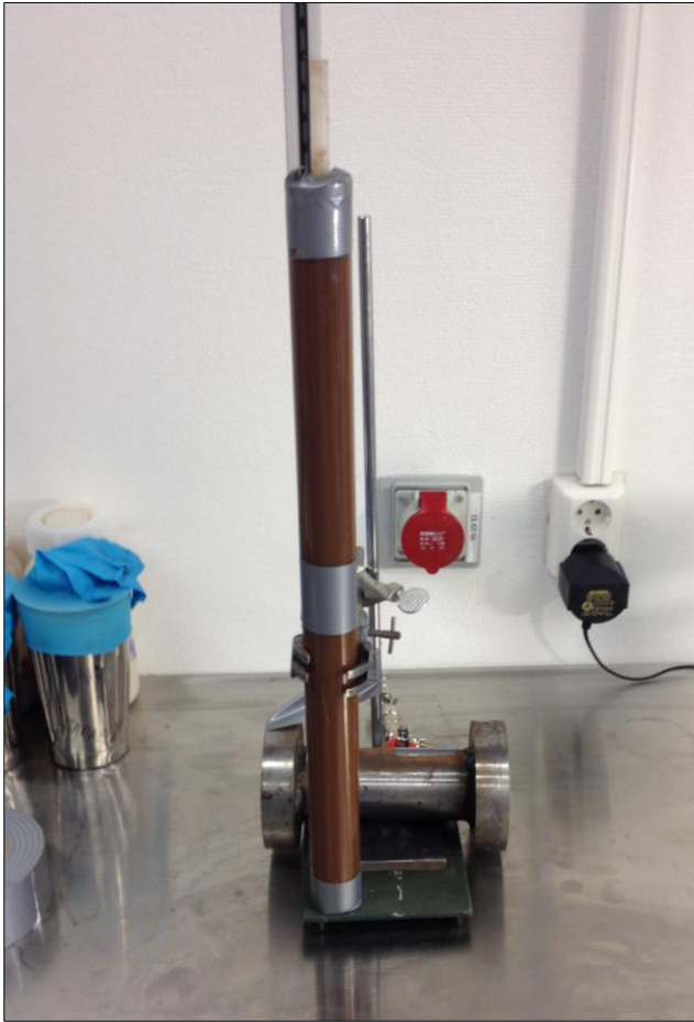
Figure 4-9: Horizontal section sag test – filling of drilling fluid. [P1]
