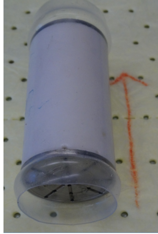
(a) Visible hole in the sleeve at the inlet side of the core.
