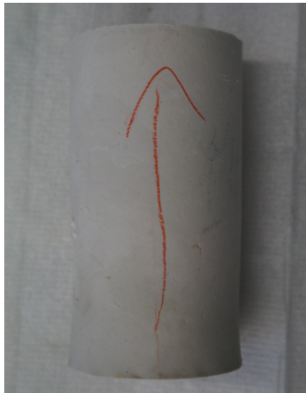
Figure 4.8: Picture of Mons core M6 showing permanent deformation after testing. The arrow indicate flooding direction during testing.
