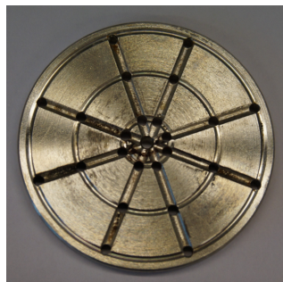
(a) Flooding holes close to the edge.
