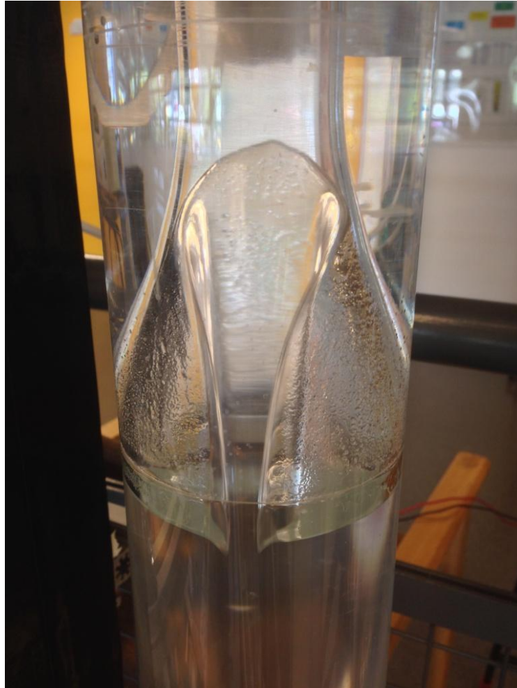
Figure 31. Fluid creates a channel in bubble in flow rates related to 12 v.
