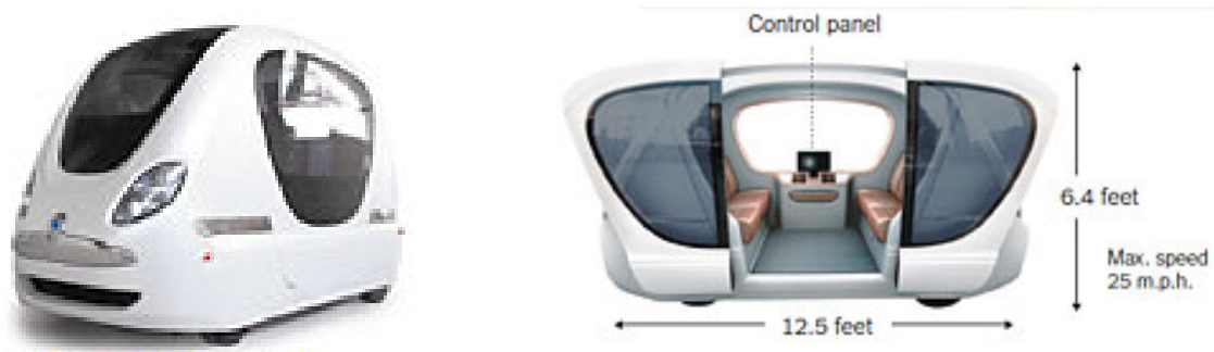
Figure 3.9: Personal Rapid Transit (PRT) vehicle with measurements (Kimball, 2010)
