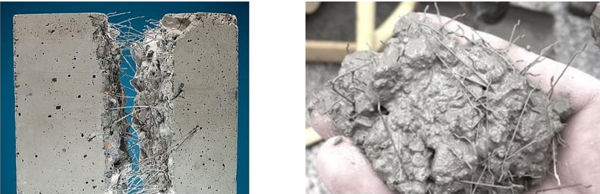
Figure 1 – Steel fiber in concrete (Mahajan, 2022)
