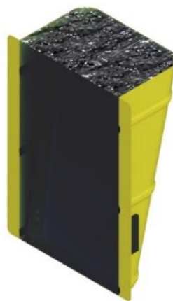
Figure 4 - 8 GRP cover with trapped water from Autodesk Inventor.
