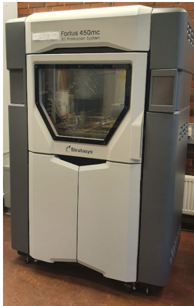
Figure 4-16 - Fortus 450mc (Industrial FDM 3D printer at UiS)
