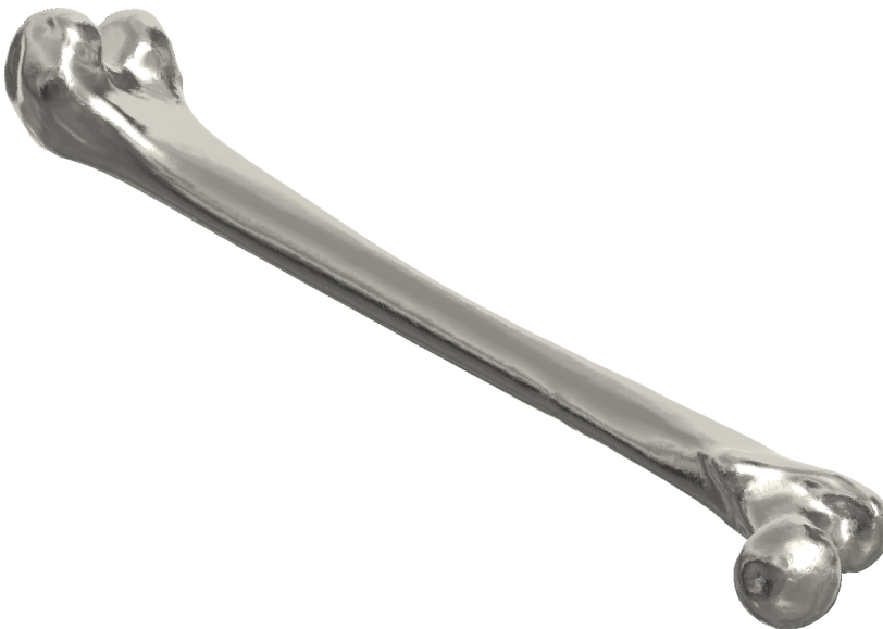
Figure 5-4 - Handyscan 700 model converted directly to solid in Autodesk Inventor
