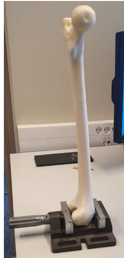
Figure 4-32 – 3DP model setup of femur for scanning (Einscan HX)
