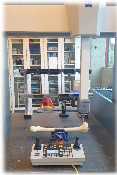
Figure 4-24 - Scanning of femur using CMM
