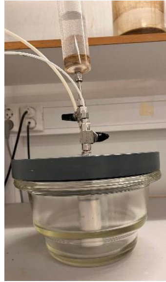
Figure 3.1: Vacuum chamber used to saturate the cores
