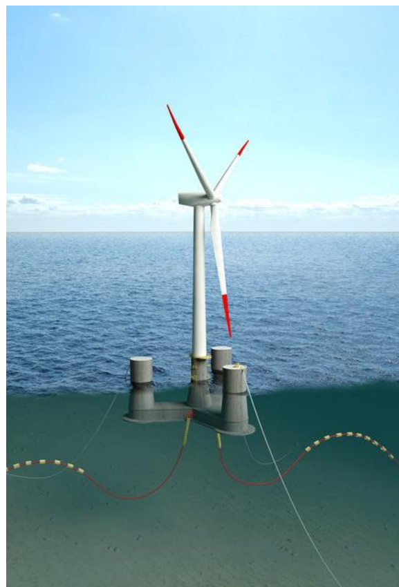
118 Figure 1 The LIFES50+ OO-Star Wind Floater Semi 10MW structure [37].
