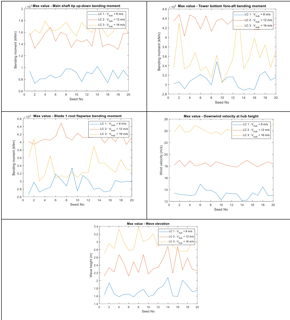
Figure 49 Maximum value in each realization. Figures Identity - Top-left: LSSTipMys; Top-right: TwrBsMyt; Centre-left: RootMyb; Centre-right: Wind velocity (Downwind at hub); Bottom: Wave elevation
