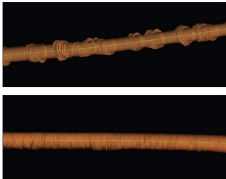
Figure 6.3 - Wellbore Quality Comparison: above – PDM, bottom – RSS
