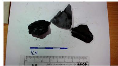
(c) Mechanical, angular slightly rounded cavings showing weak bedding planes found at 21380 ft MD
