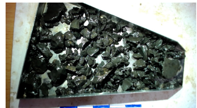
(f) Small tabular and sub-blocky cavings found at 9568 ft MD
