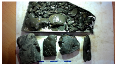
(e) Blocky and tabular, rounded to sub-rounded cavings found at 15632 ft MD
