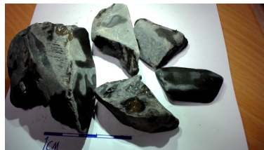
(b) Angular and tabular cavings found at 20156 ft MD
