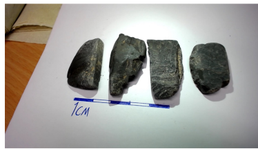
(b) Mechanical, platy, sub-angular cavings showing weak bedding planes found at 18450 ft MD
