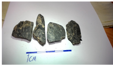
(a) Angular, platy, rounded, sub-angular cavings found at 15350 ft MD
