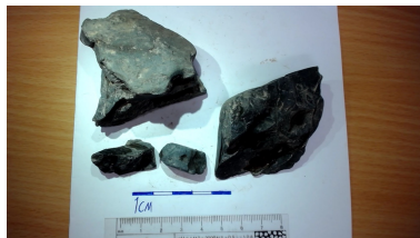
(a) Angular, slightly rounded cavings found at 20463 ft MD
