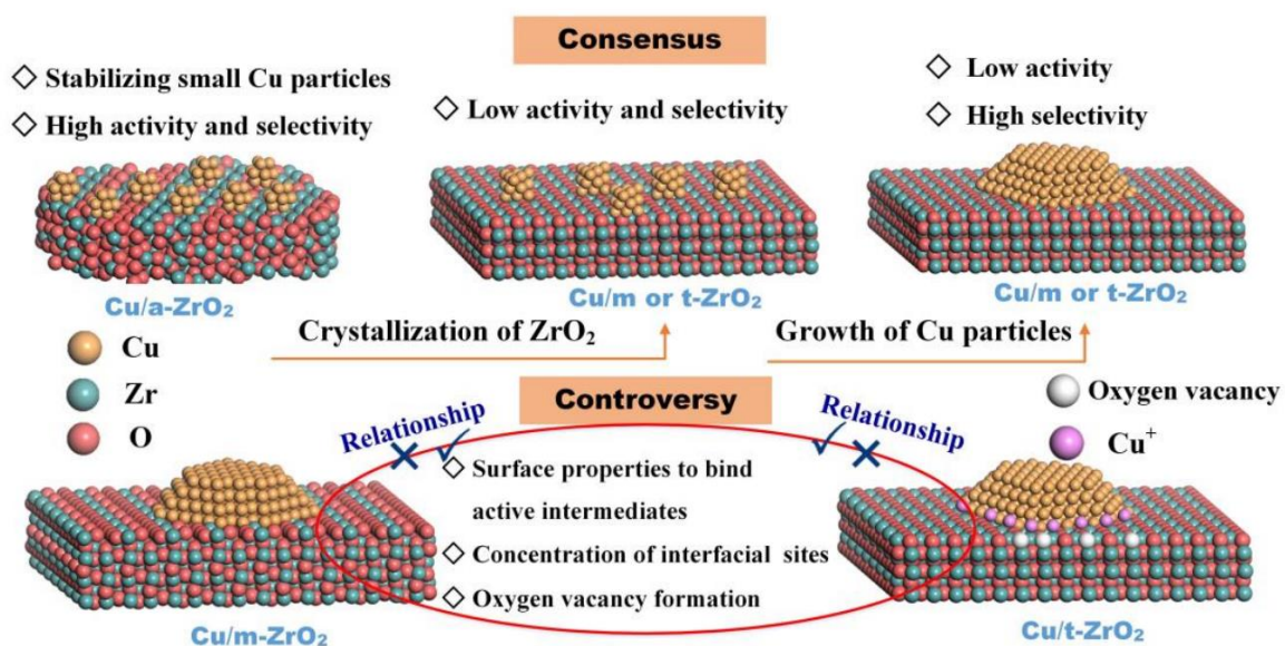
Figure 2.3: ZrO 2 phases effect on the catalytic performance [56, 59, 61].
