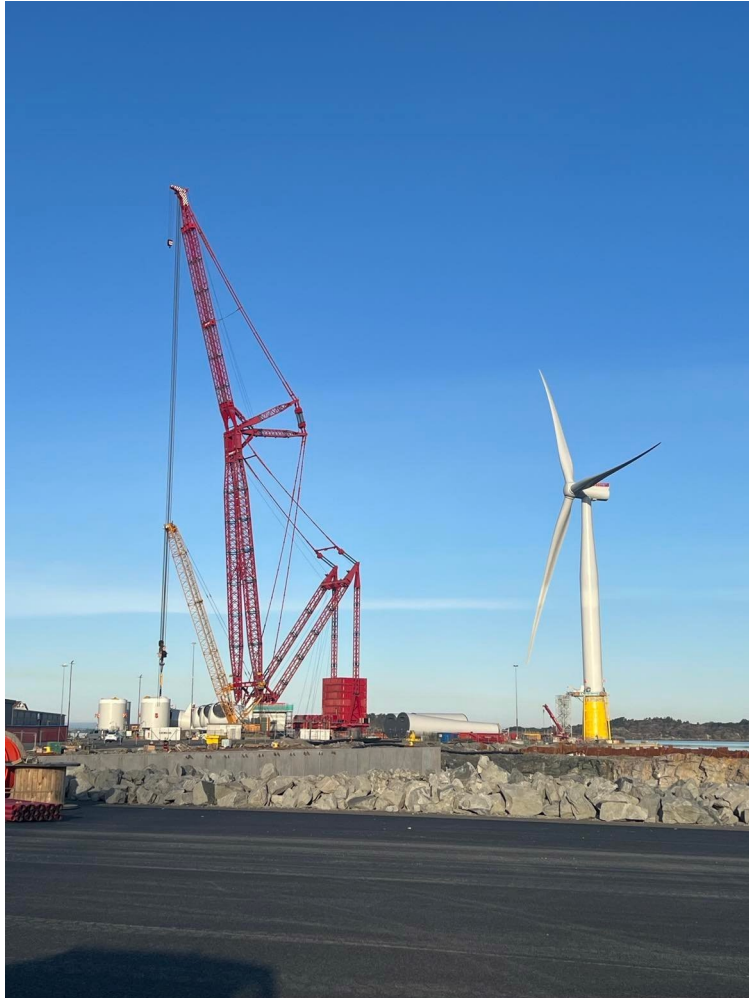
Figure 4.4.: Mammoet PTC 200-DS at the heavy lift quay at Wergeland Base, April 2022 [128]
