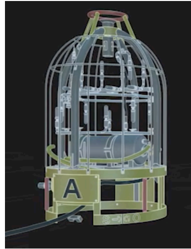
Figure 7: Subsea acoustic leak detection and condition monitoring unit (NAXYS 2015)
