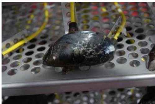
Figure 8: Instrumented blue mussels as biosensors for leak detection (Biota Guard 2015)
