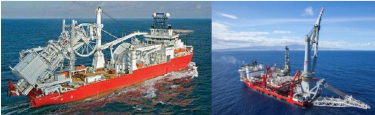
Figure 8-3 The Seven Oceans and Seven Borealis Pipe-lay Vessel, Figure from Subsea 7
