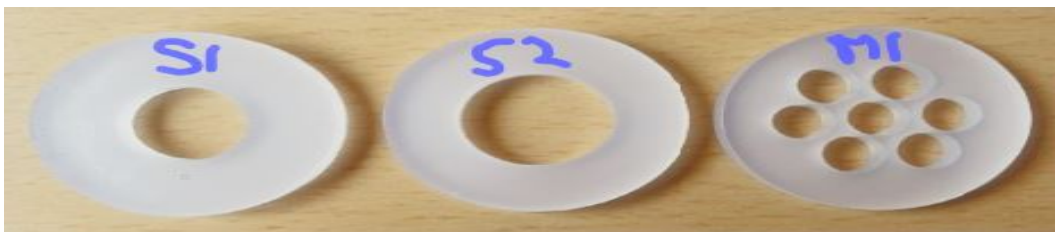
Figure 4.5: Acrylic Orifice Plates
