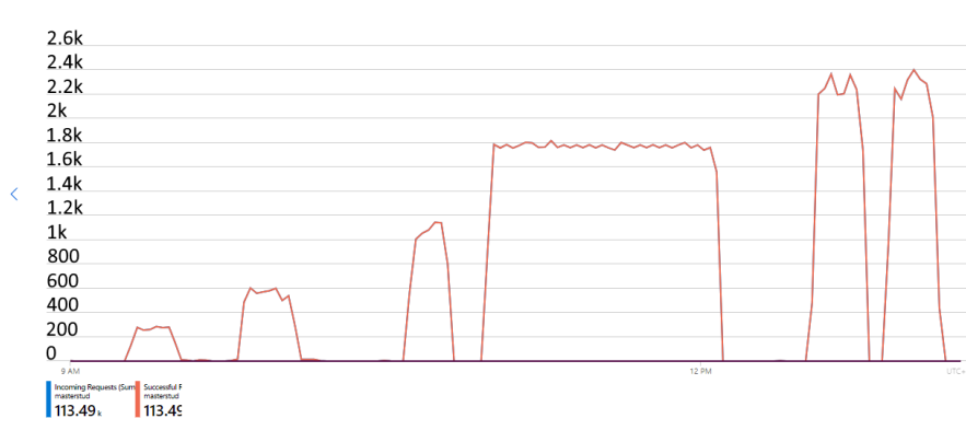
Figure 7.25: All benchmarking tests. From the left: 5, 10, 20, 60, 120 and 240 sensors
