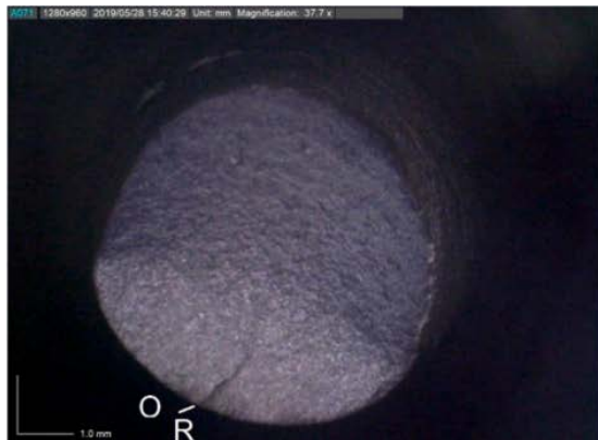
Figure 4.3 Specimen tested under \sigma_a = 207 MPa with R = 0.01 . (Dantas, 2019)
