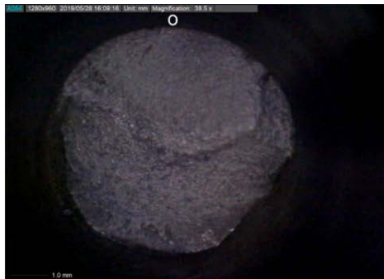
Figure 4.5 Specimen tested under \sigma_a = 168 MPa and \tau_a = 84 MPa with R = 0.01 (Dantas, 2019).
