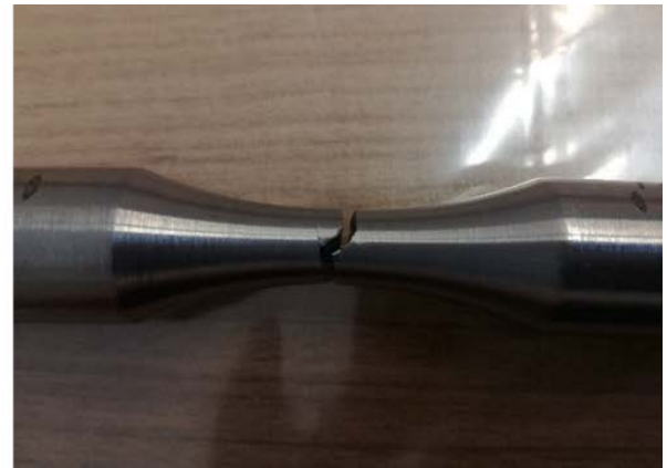
Figure 4.4 Specimen tested under \sigma_a = 272 MPa with R = -1 (Dantas, 2019).
