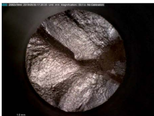
Figure 4.6 Specimen tested under \sigma_a = 204 MPa and \tau_a = 104 MPa with R = -1 (Dantas, 2019)
