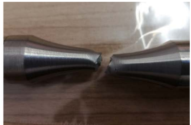
Figure 4.5 Specimen tested under \sigma_a = 168 MPa and \tau_a = 84 MPa with R = 0.01 (Dantas, 2019).
