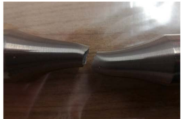
Figure 4.3 Specimen tested under \sigma_a = 207 MPa with R = 0.01 . (Dantas, 2019)
