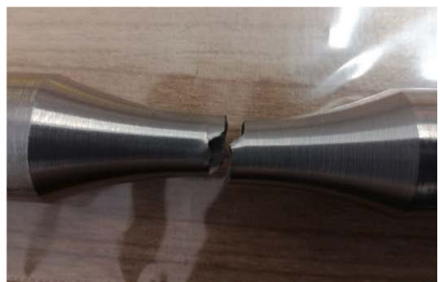
Figure 4.6 Specimen tested under \sigma_a = 204 MPa and \tau_a = 104 MPa with R = -1 (Dantas, 2019)
