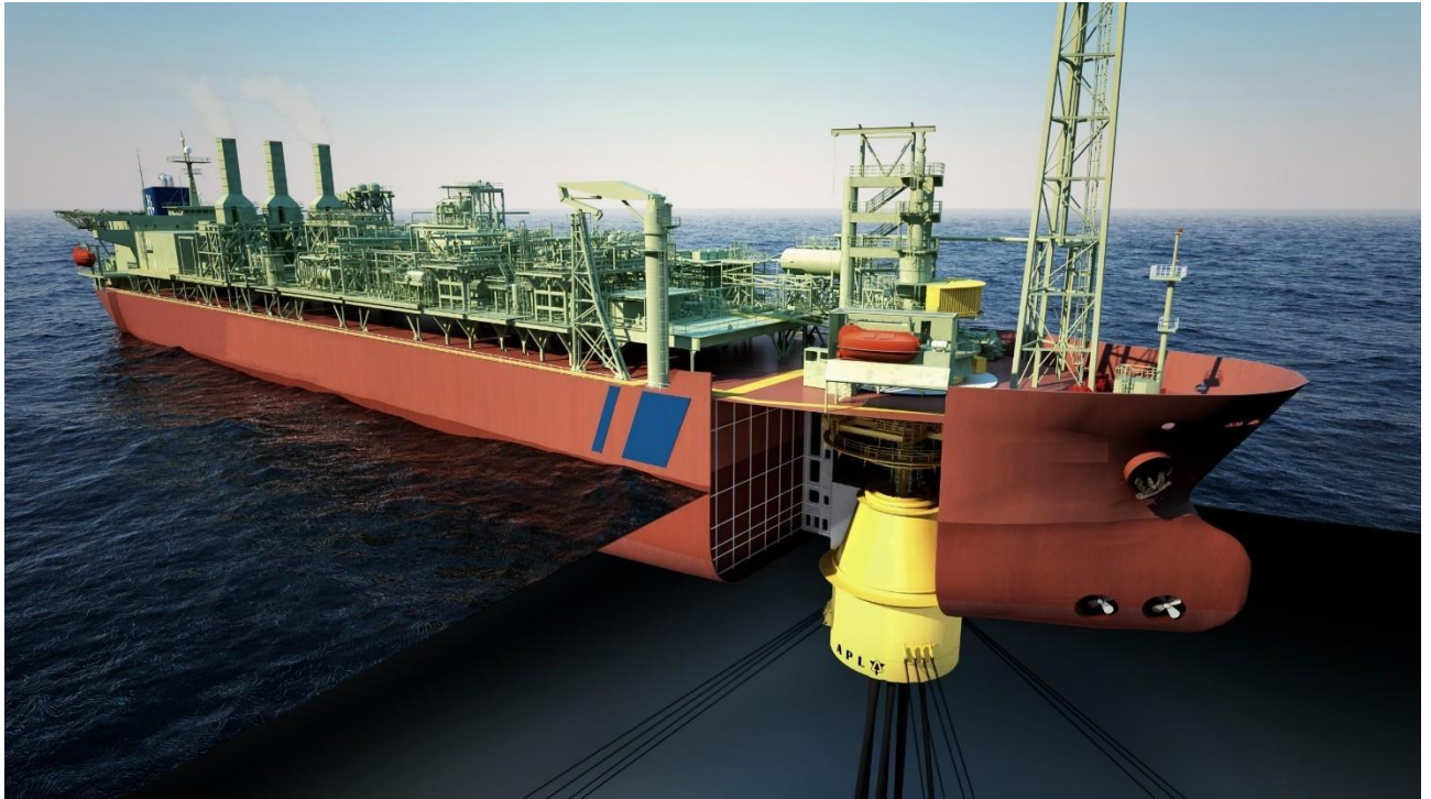
Figure 3.4 FPSO- floating systems with the ability to produce, store and unload oil.
