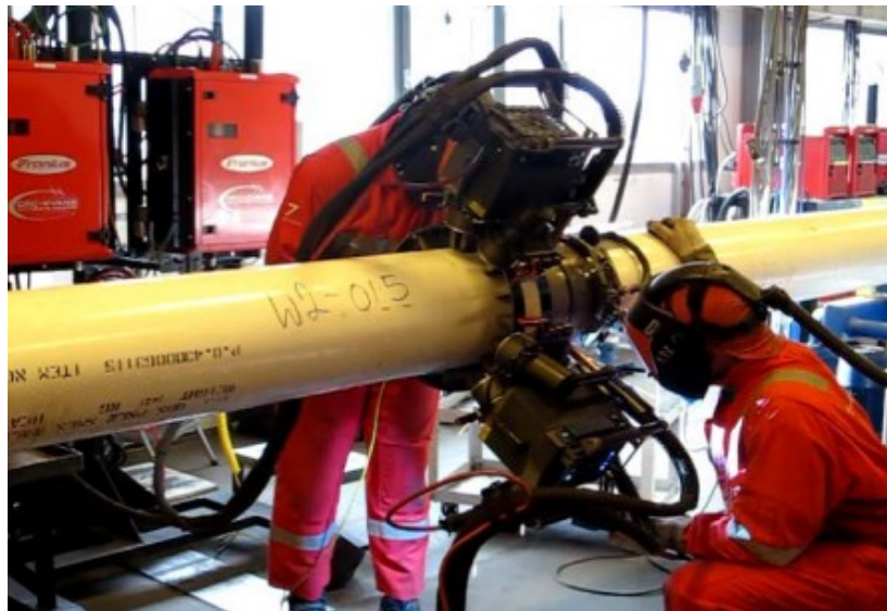
Figure 5-2: PGMAW in operation [3]
