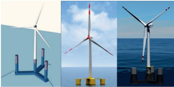
FIGURE 1: INNOVATIVE CONCEPTS OF FOWT, 5-MW-CSC (LEFT), NAUTILUS (MIDDLE), OLAV OLSEN OO STAR (RIGHT), [7]
