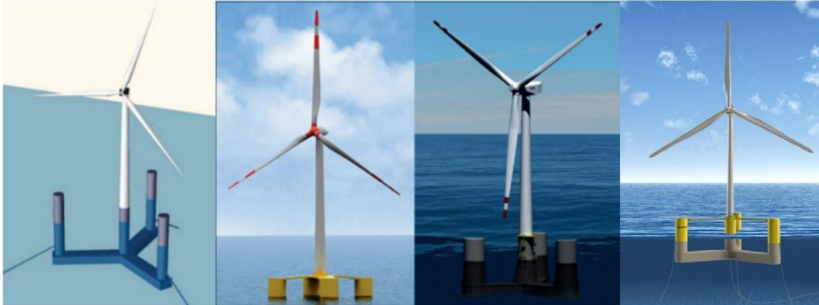
Fig. 1-2: Innovative concepts of FOWT (left to right), 5-MW-CSC, Nautilus, Olav Olsen OO-Star, UMaine VoltturnUS-S [11, 14]
