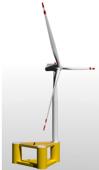
Figure 4-1 12MW WINDMOOR FOW turbine and semi-submersible concept
