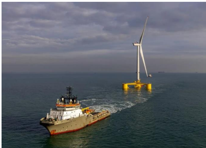
Figure 4-13 Example of tug towing semi-submersible FOW (Tomic, 2020)
