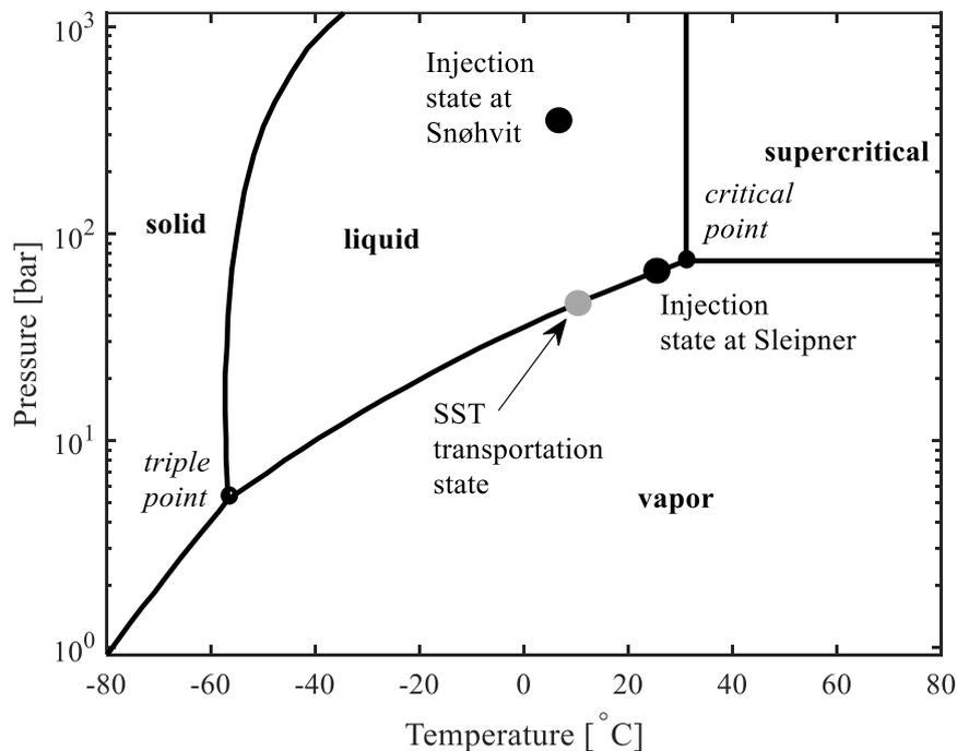
**Fig. 3.3.** CO<sub>2</sub> phase diagram with corresponding CO<sub>2</sub> states of transportation methods (data from (Ma, Xing, & Hemmingsen, 2021; Ma, Xing, Ong, et al., 2021)).
