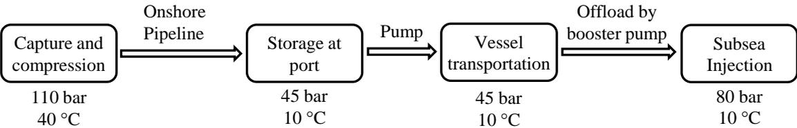
**Fig. 3.1.** CCS offshore storage process with SST transportation (Ma, Xing, & Hemmingsen, 2021).
