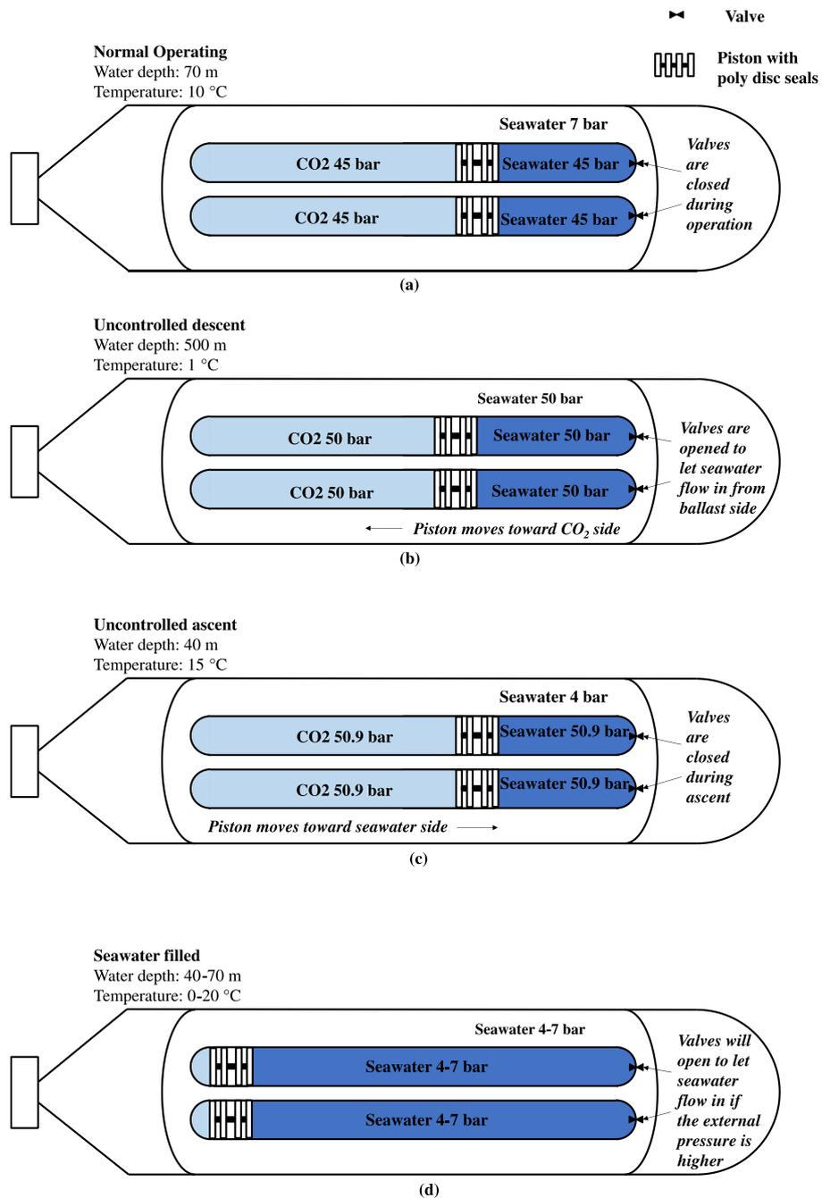
**Fig. 3.5.** Pressure compensation system.
