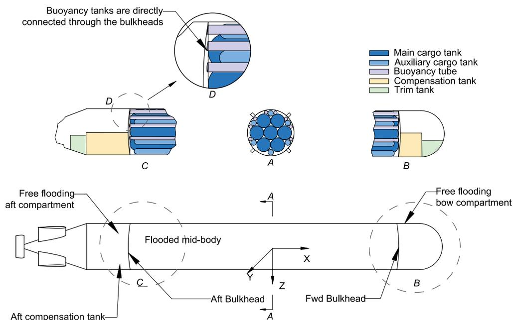
**Fig. 3.4.** SST general arrangement. A: Mid-vessel cross-section. B: SST fwd bulkhead. C: SST aft bulkhead. D: Buoyancy tank-bulkhead connection (Ma, Xing, Ong, et al., 2021).
