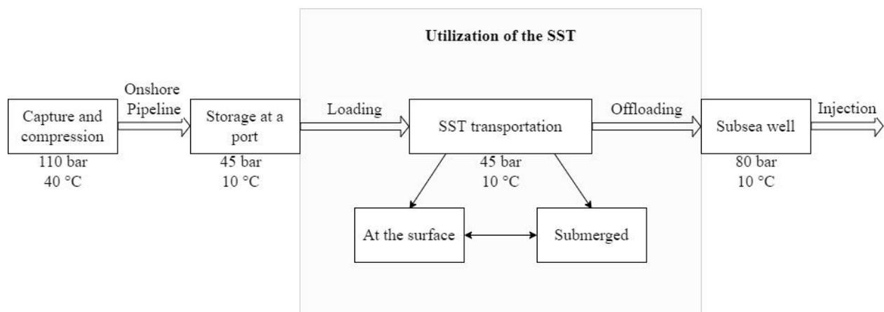
**Fig. 4.1** SST functional diagram of operational phases.
