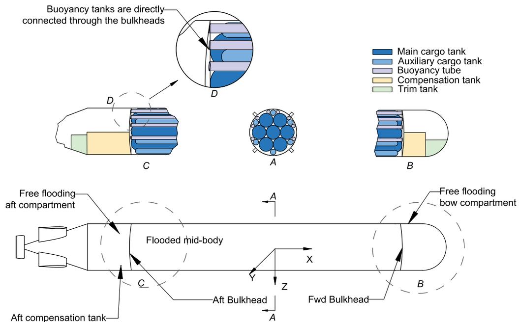
**Fig. 5.** SST general arrangement. A: Mid-vessel cross-section. B: SST fwd bulkhead. C: SST aft bulkhead. D: Buoyancy tank-bulkhead connection [7].
