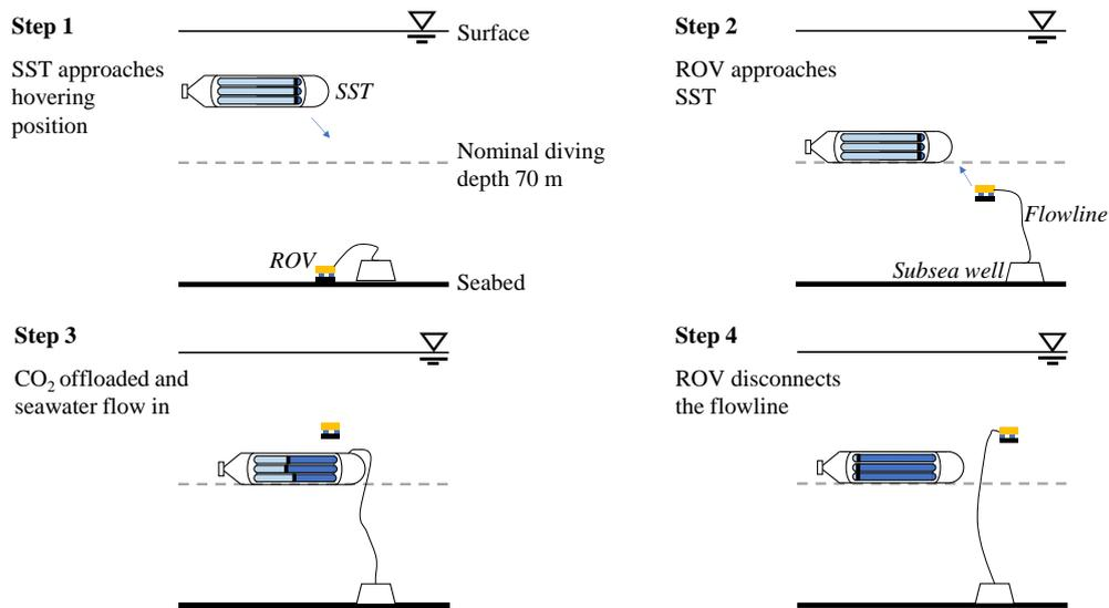
**Fig. 3.6.** SST loading and offloading procedure.
