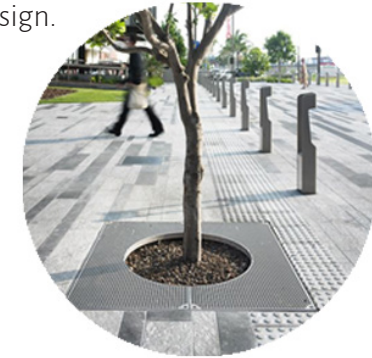
Figure 102: Sidewalks and road having same material with no height differences, providing a universal design.
