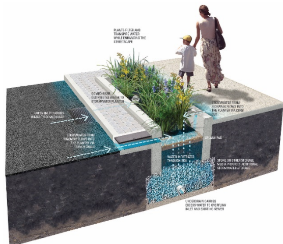
Figure 17 Stormwater Planter construction (Philadelphia Water Department. (2016))
