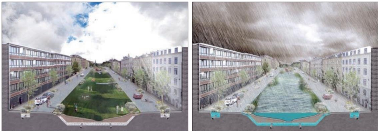
Figure 6.4. Illustration of open stormwater handling solution in Copenhagen (Aspegren, et al., 2014)
