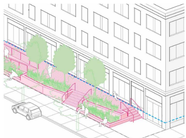
Figure 5.18. Using stairs as a flood mitigation measure (McGuinness, et al., 2019)
