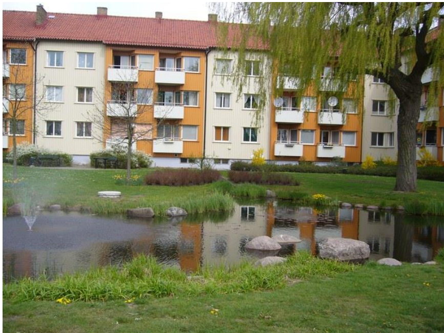
Figure 6.1. Pond in a residential area in Malmö acting as a water catchment area (ClimateAdapt, 2021)
