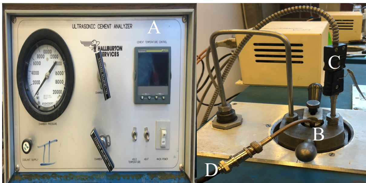
Figure 13: Halliburton Services Ultrasonic Cement Analyzer was used to measure the transit time through the slurry. A; The manifold of the UCA machine, B; UCA mold, C; temperature sensor, D; electric signal sensor.
