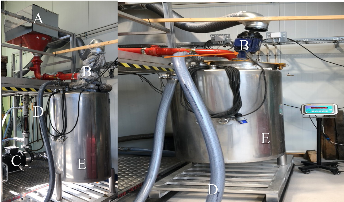
Figure 4: The main components of the NORCE mixing unit; A: dry material inlet, B: agitator, C: circulation pump, D: return line of the circulation loop, E: mixing tank
