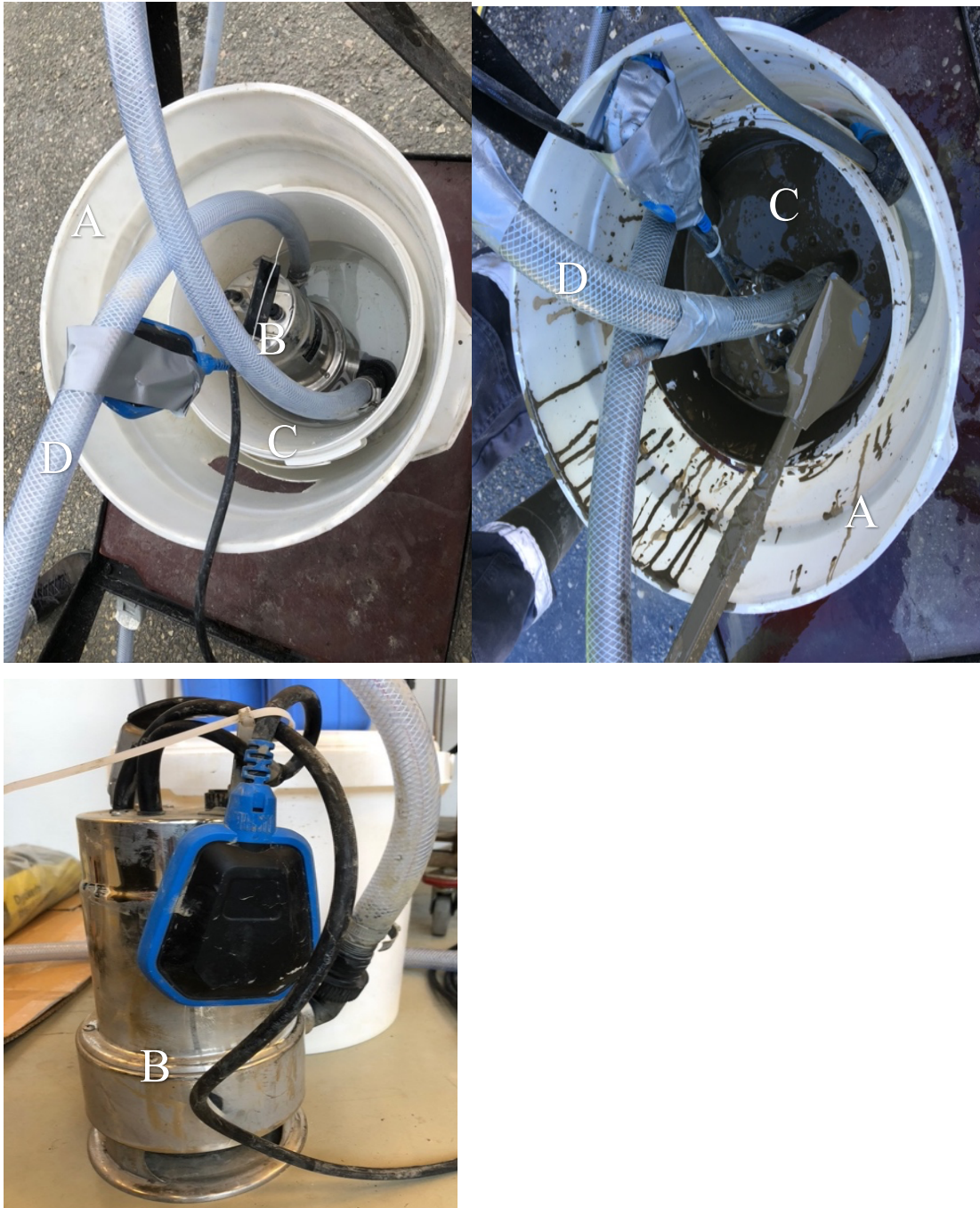
Figure 9: The 15 liters mixing unit. A: Cooling tank, B: Pump, C: Mixing tank, D: Circulation loop.
