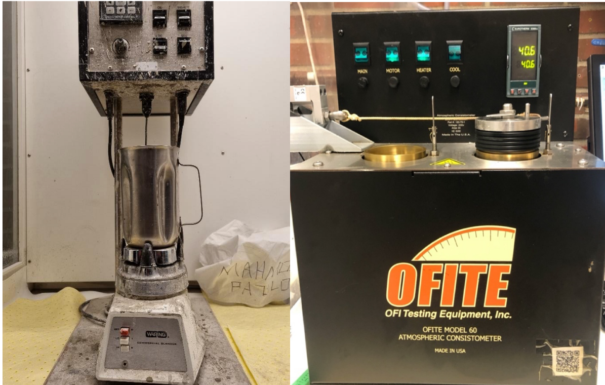
Figure 7: Left; Waring blender used for mixing the cement slurry in the laboratory, Right; Ofite Model 60 atmospheric consistometer used to condition the cement slurry in the laboratory.
