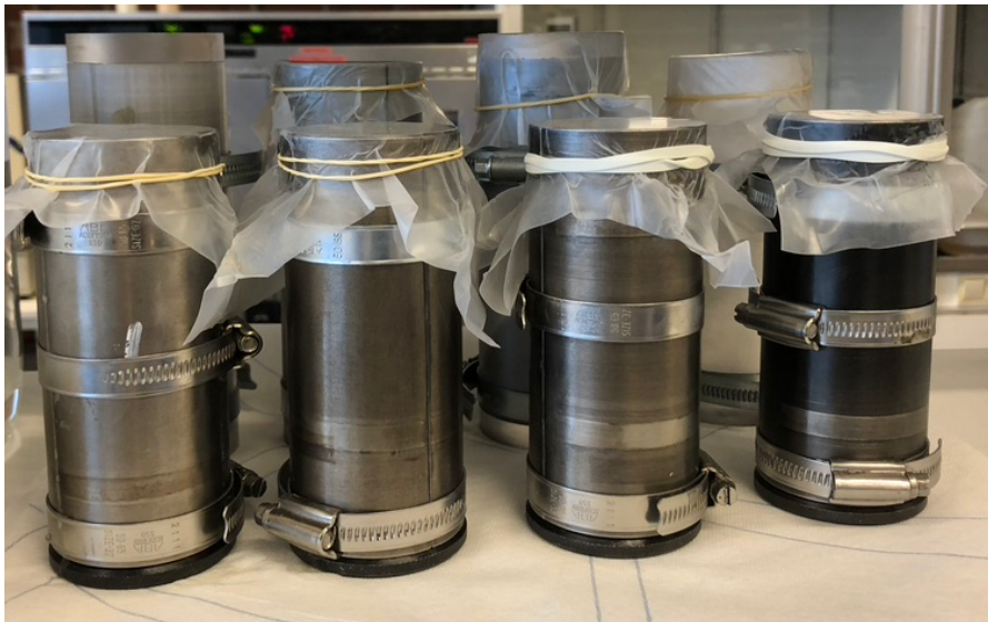
Figure 15: Metal molds (in the front) and 3D printed plastic molds (in the back) used to cure samples for UCS and Young's modulus measurements.
